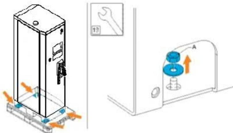
9. Remove the nuts (A) at the four corners.
