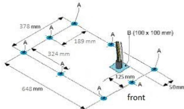
1. Drill and tap 8 holes (minimum recommended 3/8" or M10, 5/8" is common) in the floor at the indicated positions (A), depth  $\pm 60$  mm.
