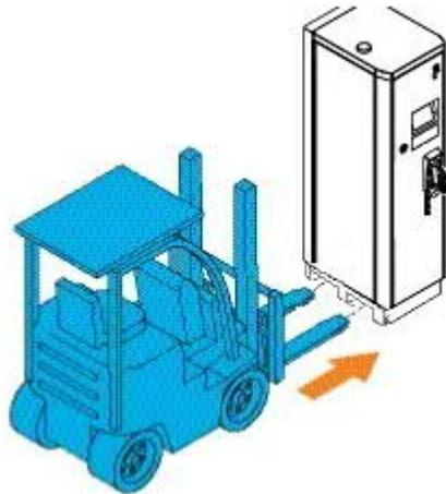
1. Move the forks of the forklift truck in the gaps at the side of the Terra 54.
