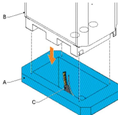
Placement on a concrete foundation
