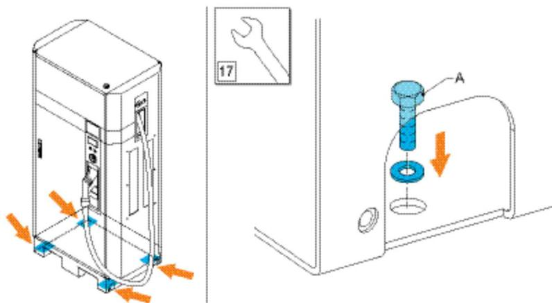
4. Insert bolts (A) and washers at the four corners and in the middle of the sides.
