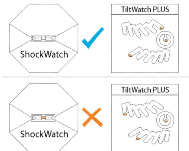
Checking the Shockwatch and TiltWatch PLUS sensors:
