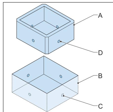
3. Prepare the site and the cable duct (D) to bring the AC wires to the location.
