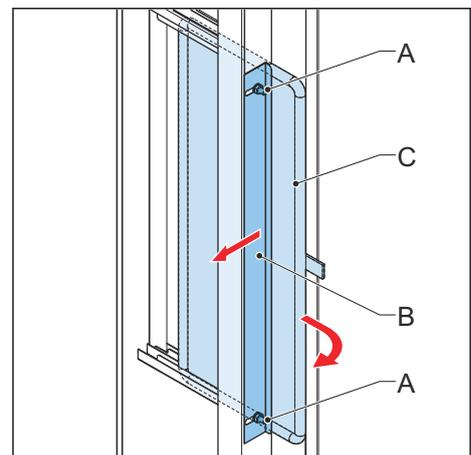
5. Carefully pull and remove the outlet filter (C).
