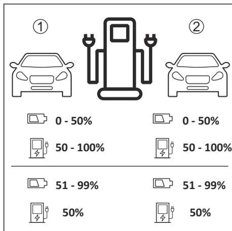
When the EVSE is configured for Fair Share power allocation, it can serve two EVs at a time with DC fast charging.
