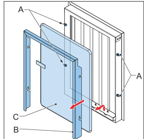
5. Install the new air inlet filter. Make sure that the air flow direction that is indicated on the air inlet filter corresponds with the air flow.
