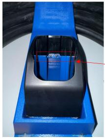
Remove the two fixing screws on the upper end of the CCS1 gun holder.
