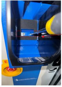
Remove the two fixing screws at the lower end of the CCS1 gun holder.
