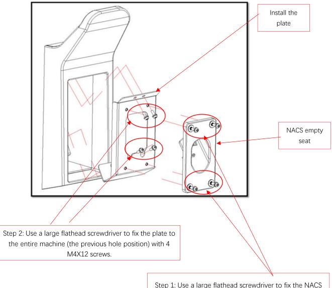
Step 1: Use a large flathead screwdriver to fix the NACS empty seat to the plate with 4 M4X20 screws.
