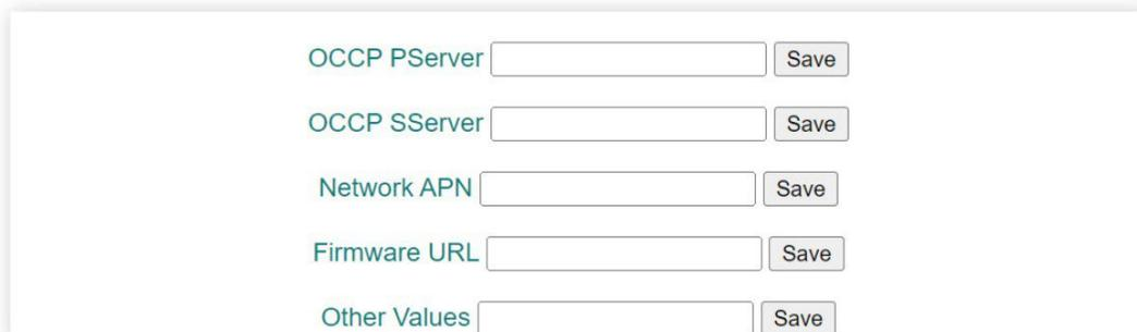
The screenshot shows a configuration web page with five rows of input fields. Each row consists of a label in teal text, an empty text input box, and a 'Save' button. The labels are: 'OCPP PServer', 'OCPP SServer', 'Network APN', 'Firmware URL', and 'Other Values'.
