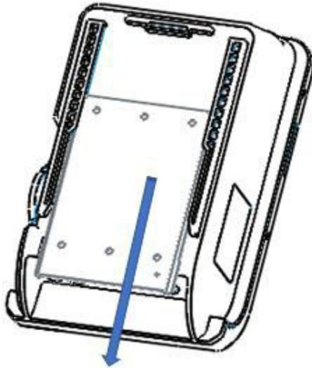
Figure 1-5 Remove the mounting bracket
