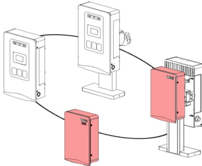
Note: The products marked in red are off grid distribution boxes, which can be ordered and installed when the off-grid function is required.
