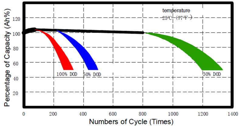
Figure 2-2: Life Cycle of the backup battery (24V)
