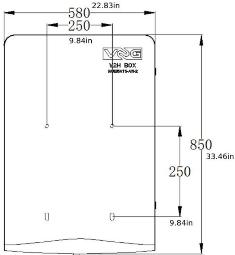
Figure 4-6: V2X Off Grid Box Back Hole Dimensions
