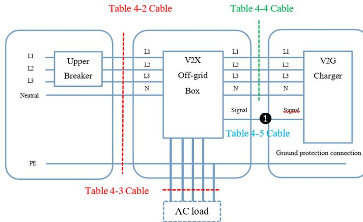
Table 4-2: AC input wiring cables chosen for V2X Off-grid Box
