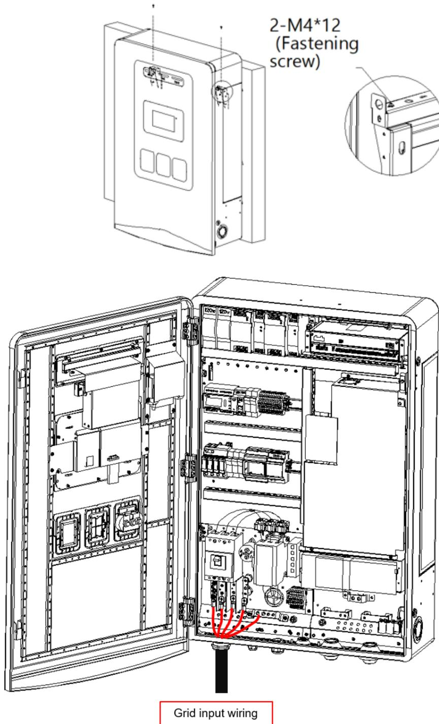
Figure 4-4: Grid Input Wiring
