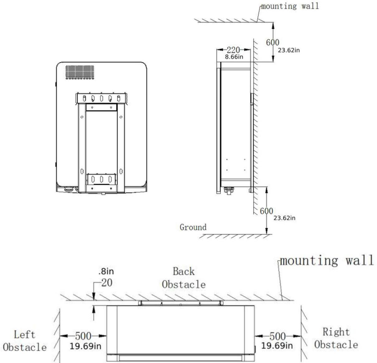
Figure 4-5: V2X Off Grid Box Space Requirements
