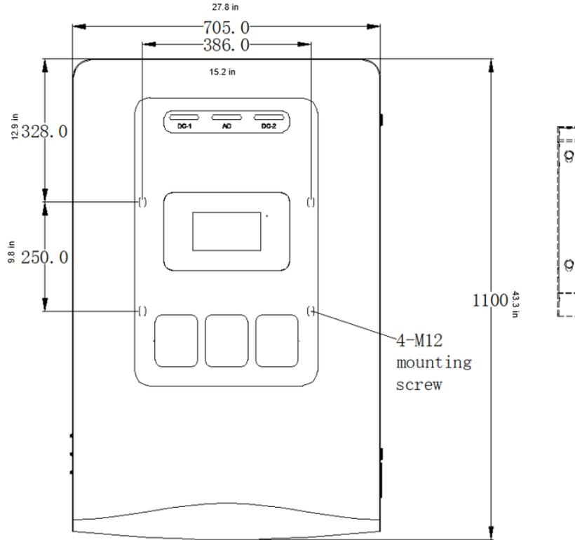
Figure 4-2: ICE-44 V2X Back Hole Dimensions
